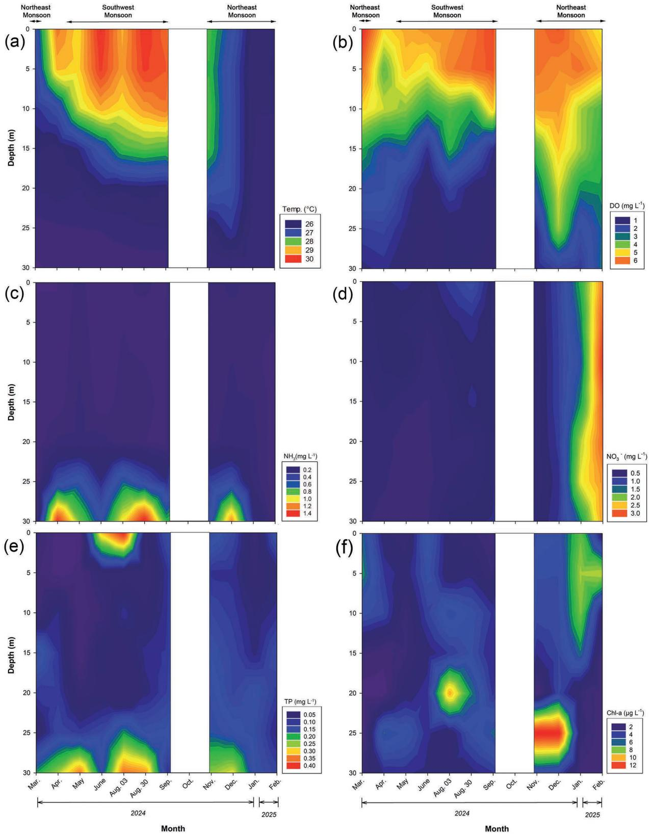
**Fig. 3.** Monthly vertical profiles of temperature (a), dissolved oxygen (DO) (b), ammonia (NH<sub>3</sub>) (c), nitrate (NO<sub>3</sub><sup>-</sup>) (d), total phosphorus (TP) (e), chlorophyll-a (Chl-a) (f) from March 2024 to February 2025.
