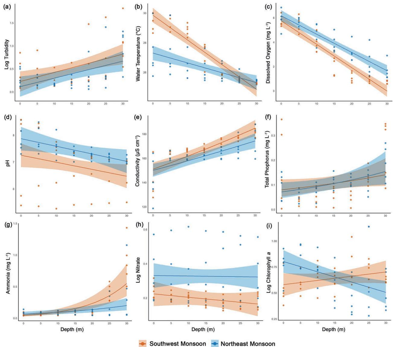
**Fig. 2.** Seasonal variation in environmental variables across depths modeled using mixed-effects analyses. a) Log turbidity; b) temperature; c) dissolved oxygen; d) pH; e) conductivity; f) total phosphorus; g) ammonia; h) log nitrate; i) log chlorophyll-a. Shaded areas show 95% confidence intervals.
