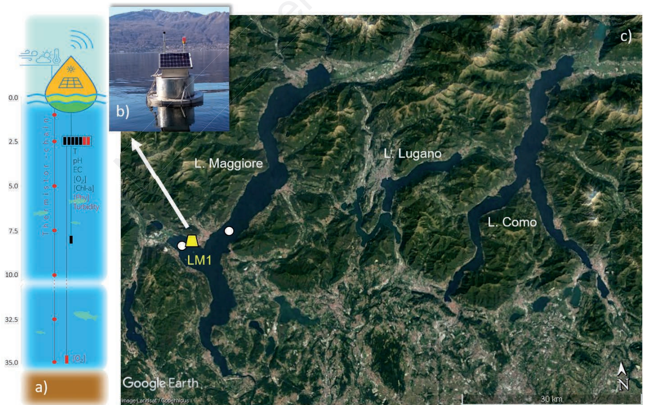
Fig. 1. LM1. a) Description of the main components of LM1, parts in red are projected, not yet present components. b) LM1 buoy. c) Location of LM1 and of the long-term sampling stations (white dots) in Lake Maggiore.
