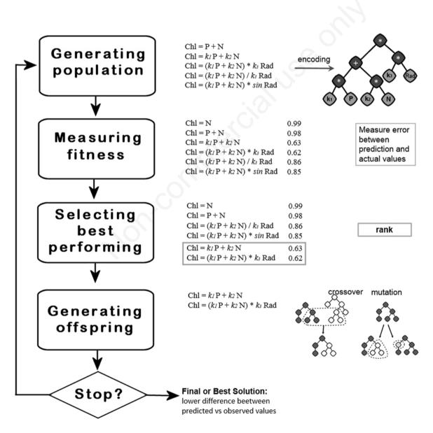
Fig. 1. Flow chart of Genetic Programming data processing.
